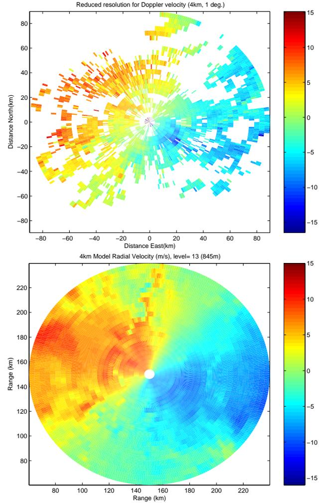
**Fig. 6.** The super-observed Doppler radial winds, at 4 km resolution compared with the model radial velocity, at 4 km resolution.
