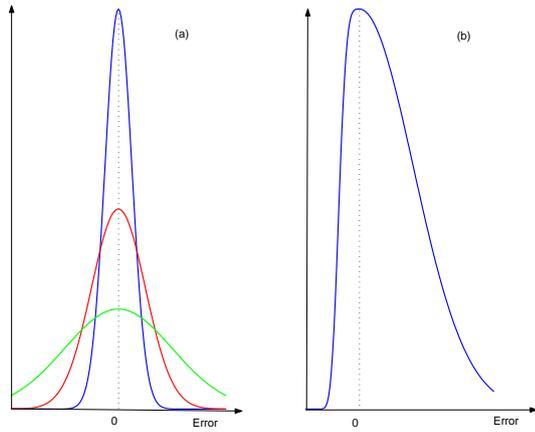
**Fig. 1.** Distribution of wind speed error due to (a) instrumental noise, and (b) strong velocity gradient across the pulse volume.
