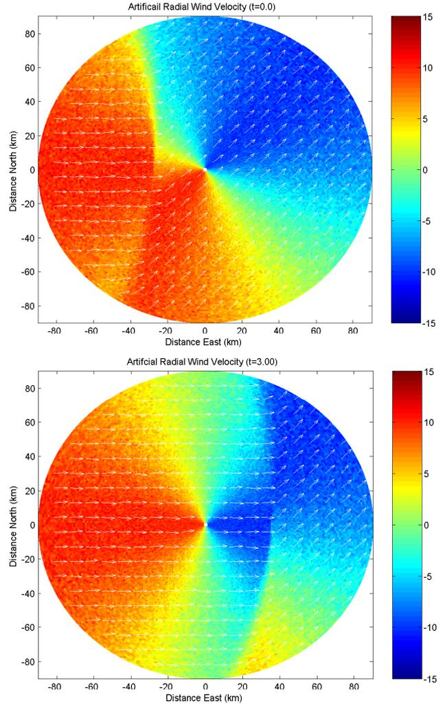
**Fig. 3.** A schematic representation of the definition of radial component of the wind field on the conical moving surface of a radar. The example shown is for a convergence line moving from the left to the right of the image. Gaussian noise has been inserted representing measurement error.
