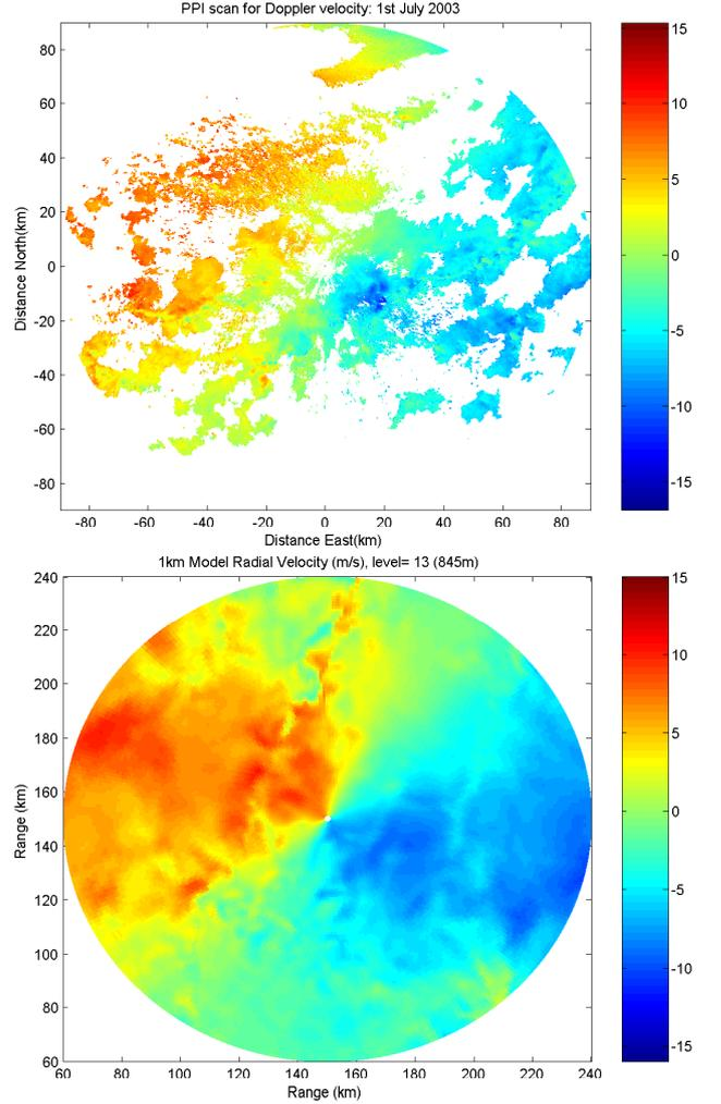
**Fig. 5.** Observed Doppler radial winds compared with the simulated model radial velocity, at 1 km resolution and model level 13, using Eq. (3).
